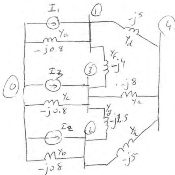
KCL (Node 1)  $I_1 = Y_a V_1 + Y_f (V_1 - V_3) + Y_d (V_1 - V_4)$
