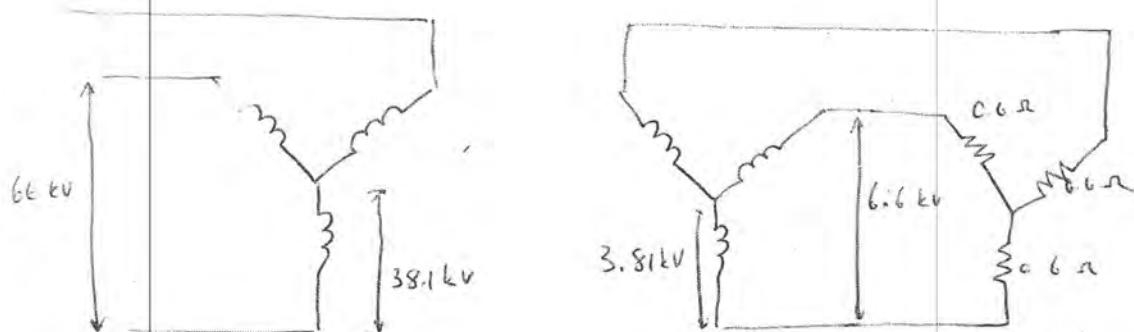
0.6  $\Omega$ /phase load is connected Y also.
