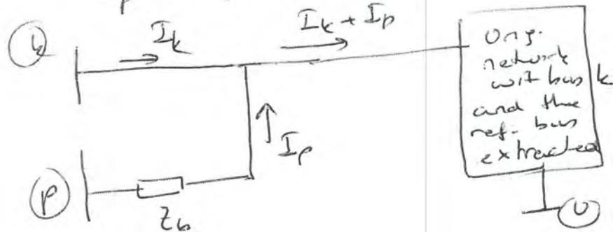
$$V_{k(\text{new})} = V_{k(\text{orig})} + I_p z_{kk}$$
