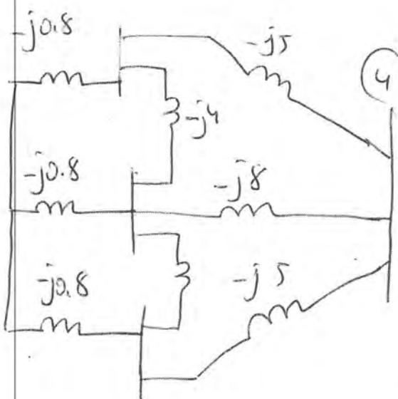
$$V_4 = Z_{41} I_1 + Z_{42} I_2 + Z_{43} I_3 + Z_{44} I_4$$
