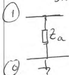
$$V_1 = I_1 Z_a \quad : \text{can be considered as a matrix eqn.}$$
